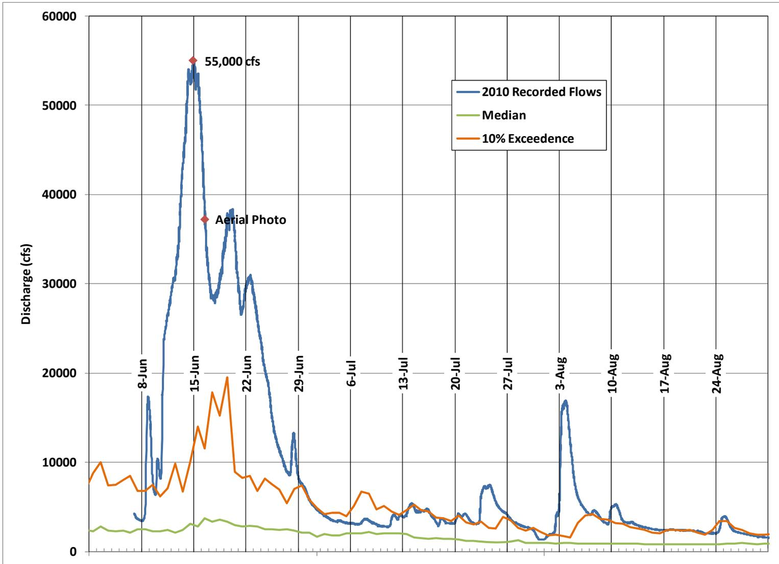
Figure 6. Provisional 2010 high flows measured at the Waterloo gage (15-minute resolution). Also shown is the peak discharge that occurred on June 14, the discharge at the time of the 2010 aerial photograph, and the median and 10% Exceedence (high) flow hydrographs for the period from WY1981 through WY2010.
