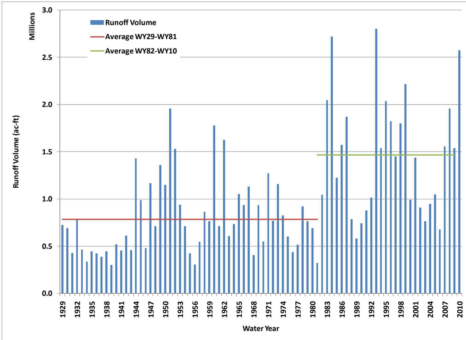
Figure 2. Annual runoff volume at the Elkhorn River at Waterloo, NE gage (USGS Gage 06800500) for the continuous period of record from WY1929 through WY2010. Also shown are the mean values for the periods from WY1929 through WY1981 and WY1982 through WY2010.
