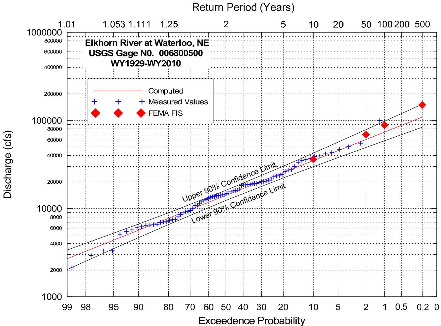
Figure 7. Flood-frequency curve for the Elkhorn River at Waterloo, based on the recorded annual peak flows from WY1929 through WY2010. Also shown are the estimated 10-, 50- and 100-year flood peaks from the Effective Flood Insurance Study (FIS) for Douglas County (FEMA, 2010) that are based on records for the period through WY1975
