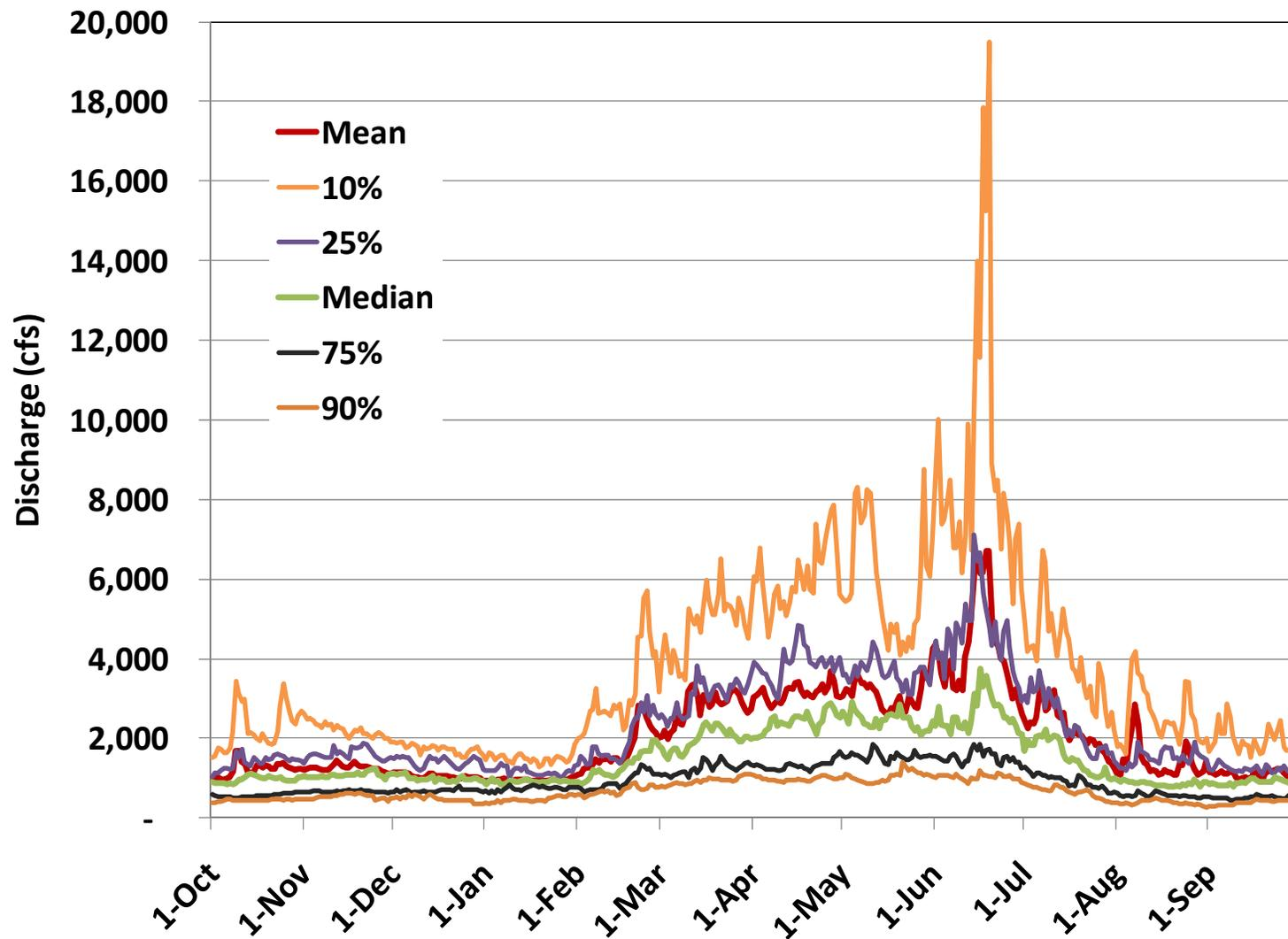
Figure 4. Mean, median hydrographs, along with the hydrographs for various exceedence percentages based on the recorded mean daily flows at the Waterloo gage during the period from WY1982 through WY2010.
